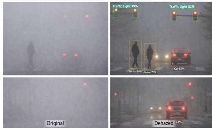
Figure 2. Sample images showing the effect of fog on object detection performance
